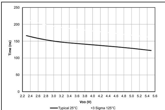
**FIGURE 38-69:** Comparator Response Time, Falling Edge, PIC16F18856/76 Only.
