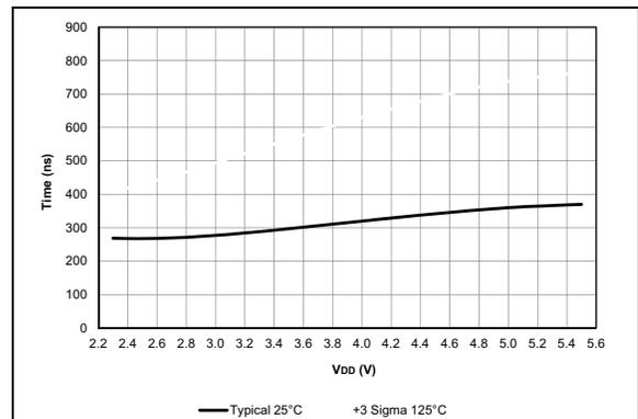
**FIGURE 38-71:** Comparator Response Time, Rising Edge, PIC16F18856/76 Only.
