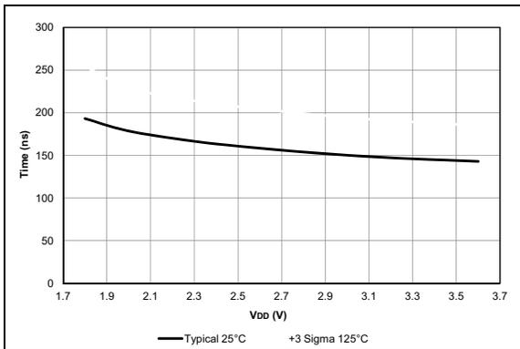
**FIGURE 38-68:** Comparator Response Time, Falling Edge, PIC16LF18856/76 Only.
