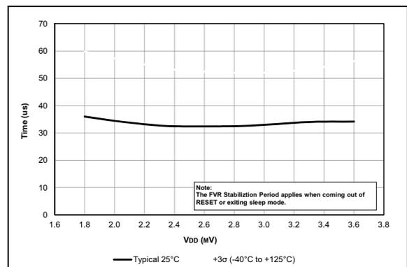
**FIGURE 38-72:** FVR Stabilization Period, PIC16LF18856/76 Only.
