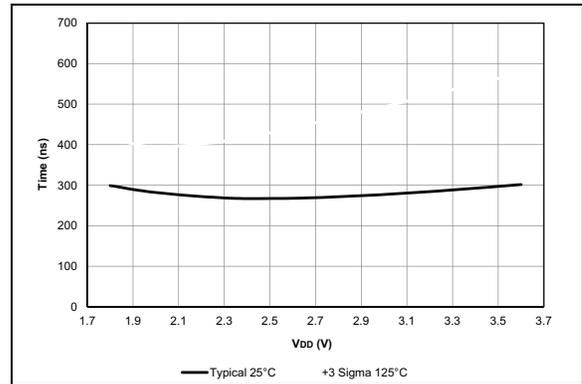
**FIGURE 38-70:** Comparator Response Time, Rising Edge, PIC16LF18856/76 Only.
