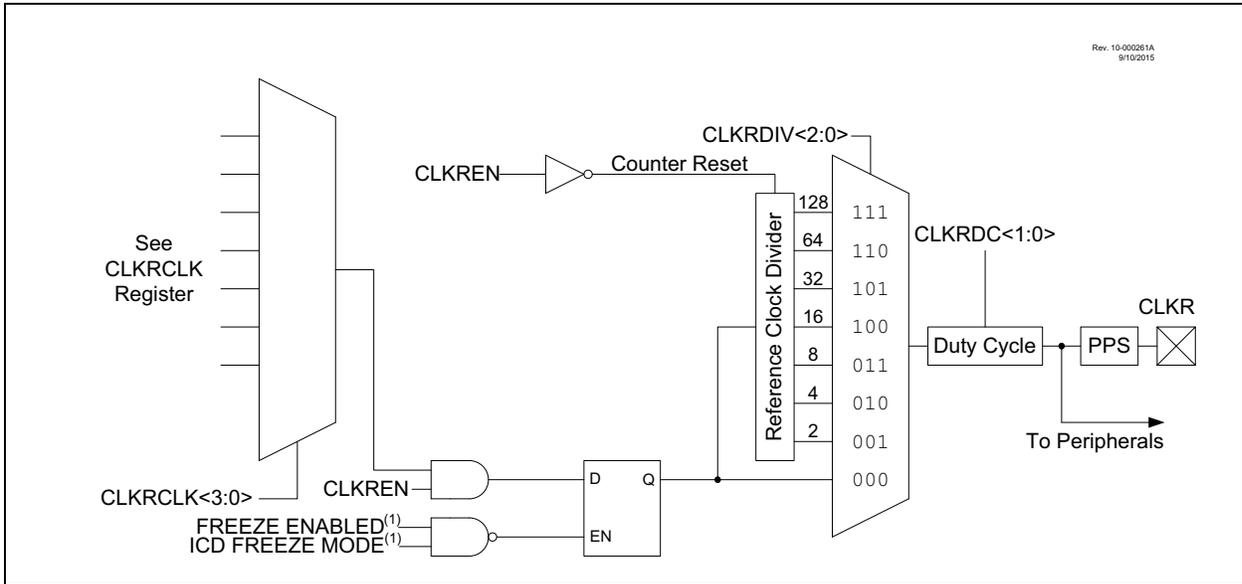
**FIGURE 34-2: CLOCK REFERENCE TIMING**
