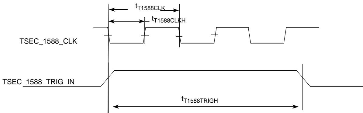
Figure 27. eTSEC IEEE 1588 Input AC timing
