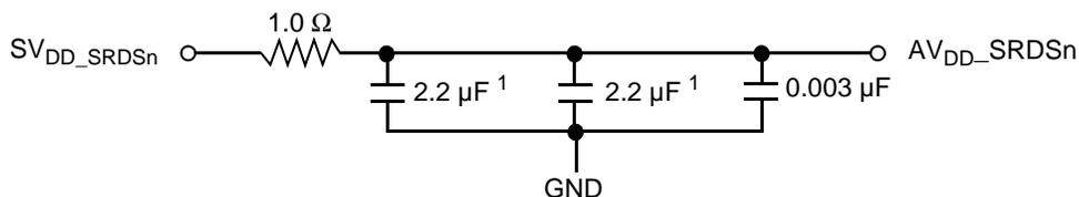
1. An 0805 sized capacitor is recommended for system initial bring-up.
