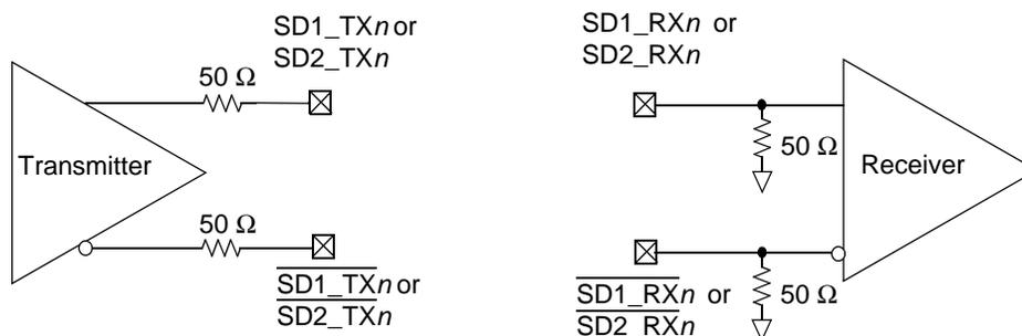
**Figure 54. SerDes Transmitter and Receiver Reference Circuits**
