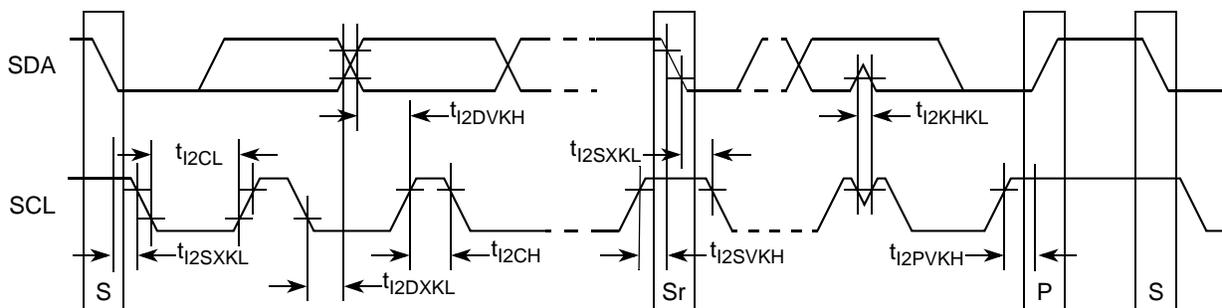
**Figure 41. I<sup>2</sup>C Bus AC Timing Diagram**
