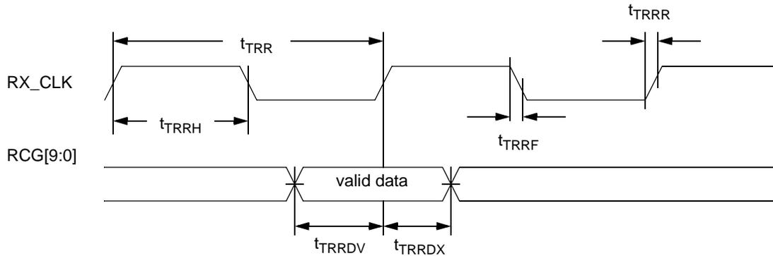
Figure 17. TBI Single-Clock Mode Receive AC Timing Diagram
