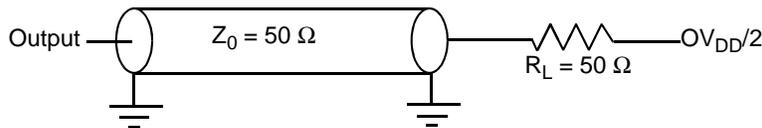
**Figure 36. AC Test Load for the JTAG Interface**
