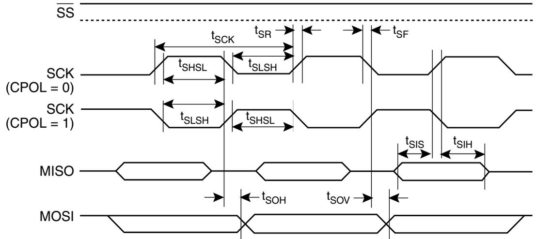
**Figure 14-8. SPI Transfer Format with CPHA = 0**
