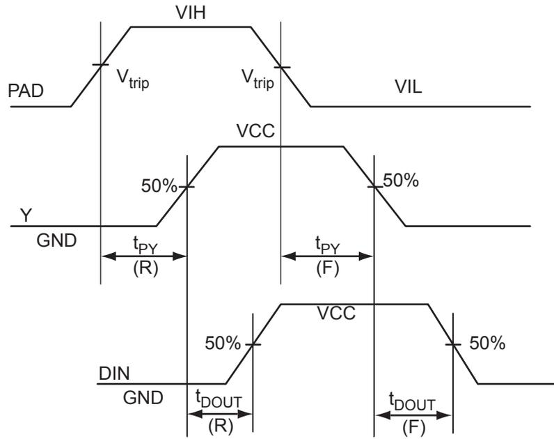
**Figure 2-3 • Input Buffer Timing Model and Delays (example)**
