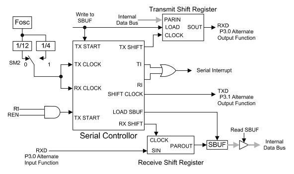
Figure 16- 1 Serial port mode 0
