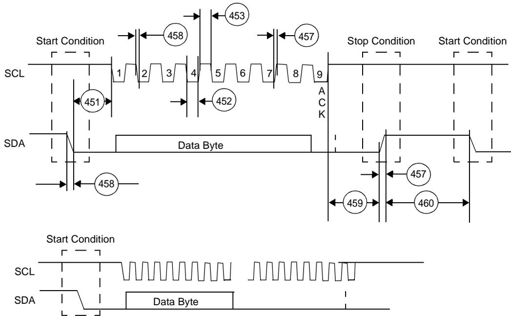
Figure 16. I<sup>2</sup>C Timing Diagram
