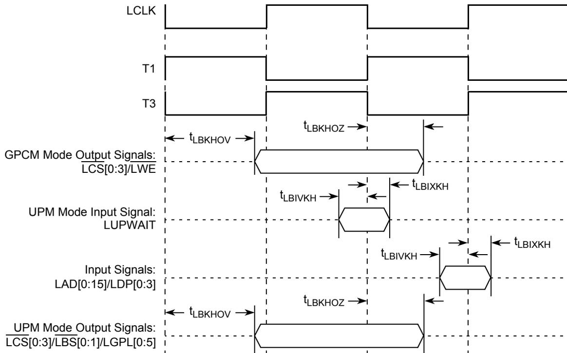
Figure 9. Local Bus Signals, GPCM/UPM Signals for LCRR[CLKDIV] = 2
