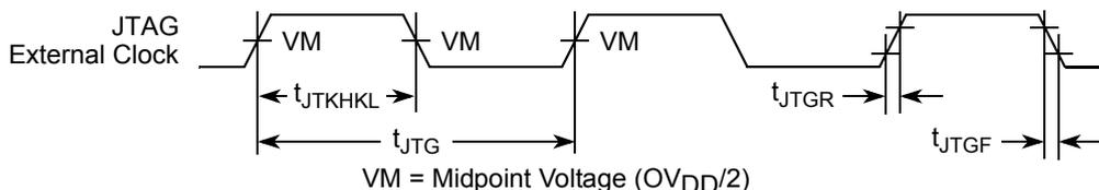
**Figure 33. JTAG Clock Input Timing Diagram**
