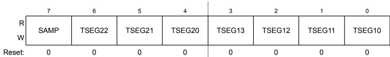
**Figure 13-7. MSCAN Bus Timing Register 1 (CANBTR1)**
