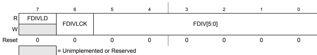
Figure 22-5. Flash Clock Divider Register (FCLKDIV)
