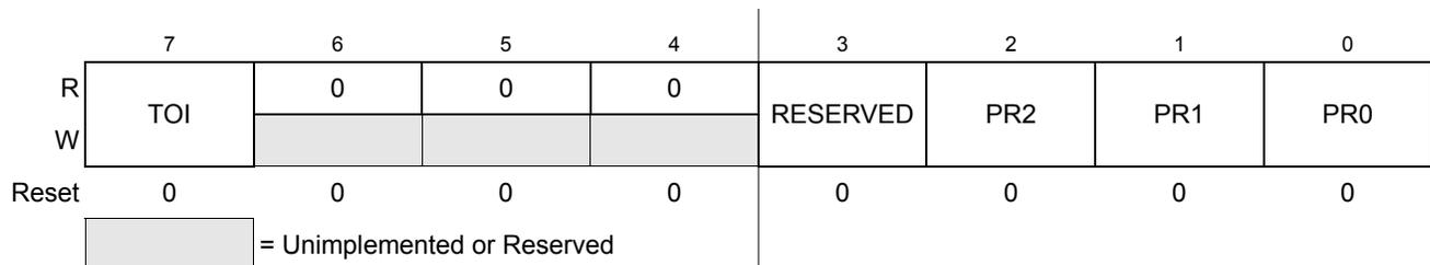
Figure 15-15. Timer System Control Register 2 (TSCR2)
