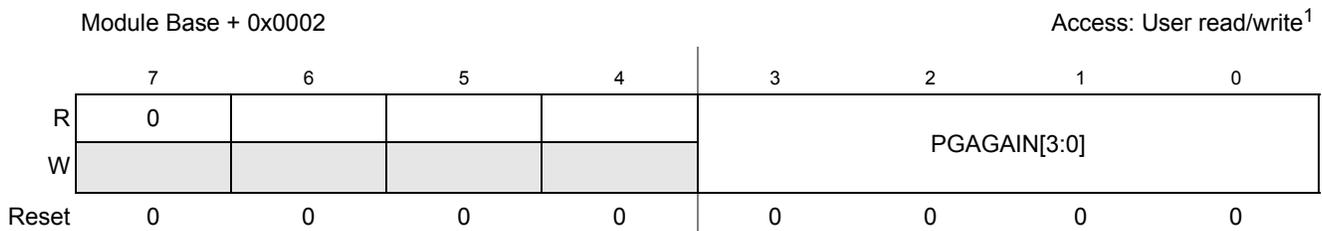
Figure 12-5. PGA Gain Register (PGAGAIN)
