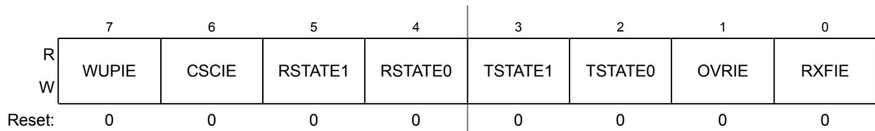
Figure 13-9. MSCAN Receiver Interrupt Enable Register (CANRIER)
