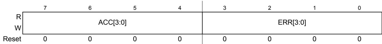
Figure 4-5. Error Code Register (MMCEC)
