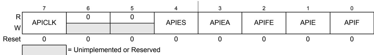
**Figure 9-22. Autonomous Periodical Interrupt Control Register (CPMUAPICTL)**
