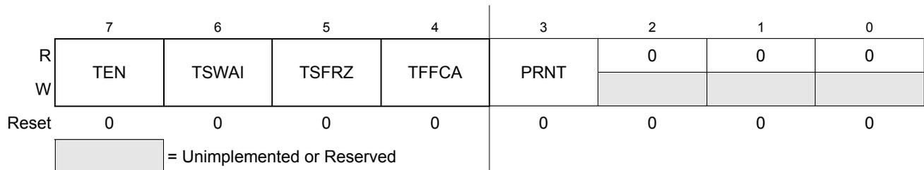
**Figure 16-8. Timer System Control Register 1 (TSCR1)**
