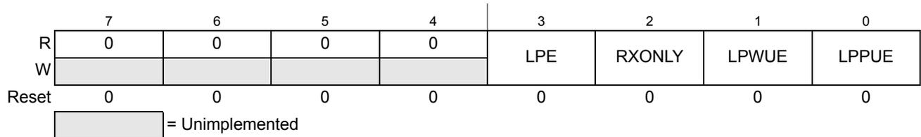
Figure 21-4. LIN Control Register (LPCR)
