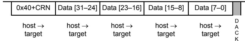
If the device is in active BDM, this command writes the 32-bit operand to the selected CPU general-purpose register. See [Section 5.4.5.1, “BDC Access Of CPU Registers](#) for the CRN details. Accesses to CPU registers are always 32-bits wide, regardless of implemented register width. If enabled an ACK pulse is generated after the internal write access has been completed or aborted.
