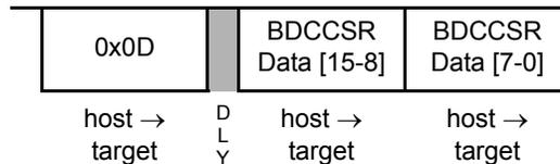
16-bit write to the BDCCSR register. No ACK pulse is generated. Writing to this register can be used to configure control bits or clear flag bits. Refer to the register bit descriptions.
