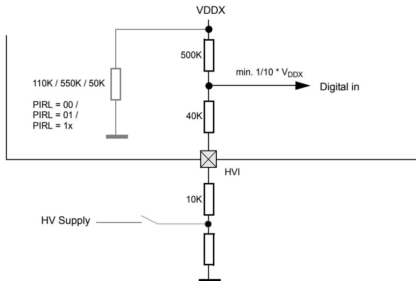
Figure 2-33. Digital Input Read with Pull-up Enabled
