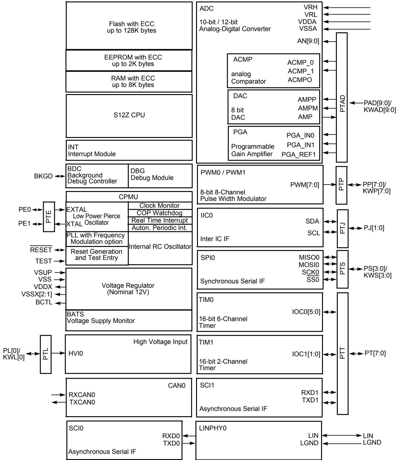
Block Diagram shows the maximum configuration
