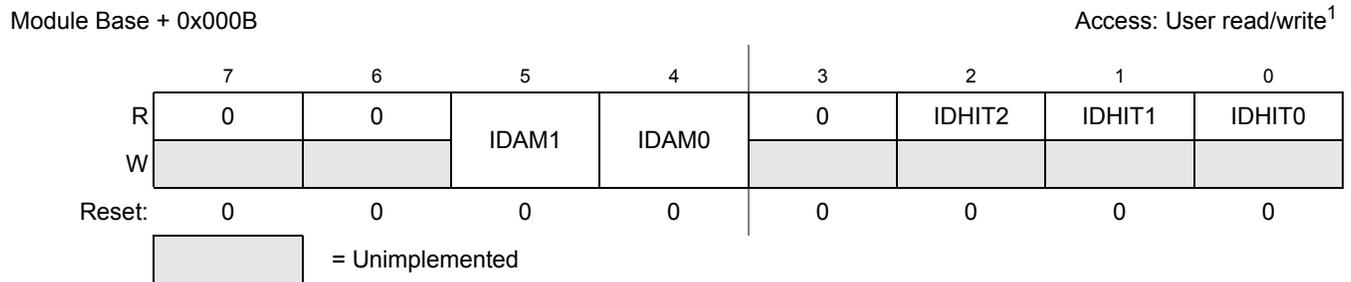
**Figure 13-15. MSCAN Identifier Acceptance Control Register (CANIDAC)**
