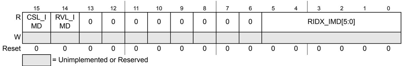
Figure 10-16. ADC Intermediate Result Information Register (ADCIMDRI)
