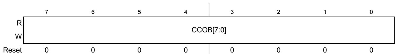
Figure 22-27. Flash Common Command Object 4 Low Register (FCCOB4LO)
