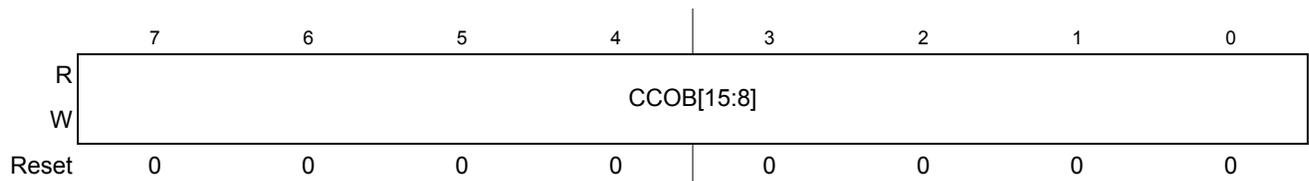
Figure 22-26. Flash Common Command Object 4 High Register (FCCOB4HI)
