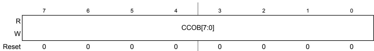
Figure 22-23. Flash Common Command Object 2 Low Register (FCCOB2LO)
