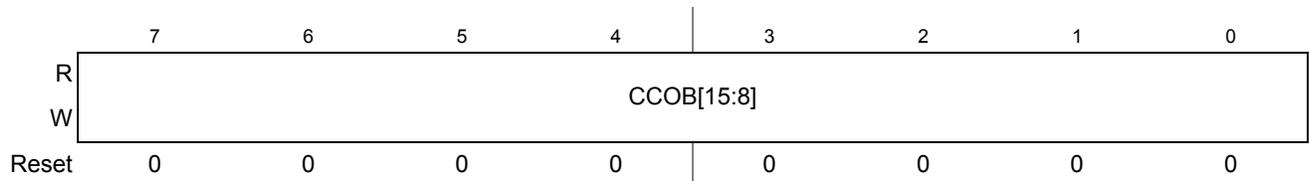
Figure 22-24. Flash Common Command Object 3 High Register (FCCOB3HI)
