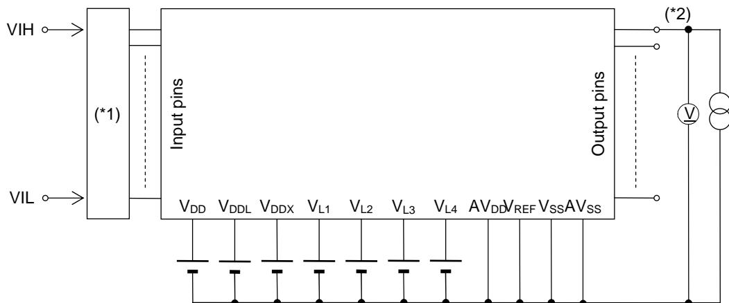
(\*1) Input logic circuit to determine the specified measuring conditions.
