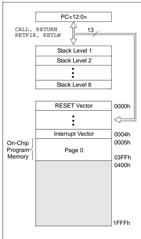
**FIGURE 2-2: PIC16C782 PROGRAM MEMORY MAP AND STACK**
