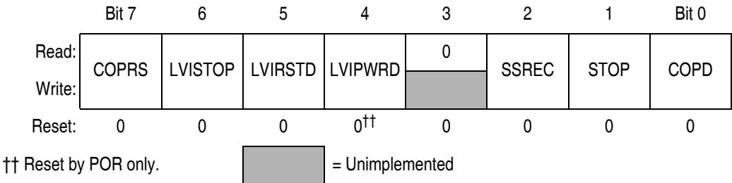
Figure 5-2. Configuration Register 1 (CONFIG1)
