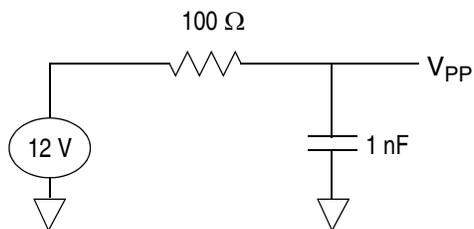
Figure 35. Example V<sub>PP</sub> Filtering
