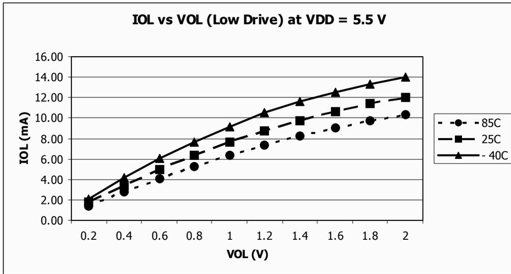
Figure 25. Typical I<sub>OL</sub> vs. V<sub>OL</sub>
