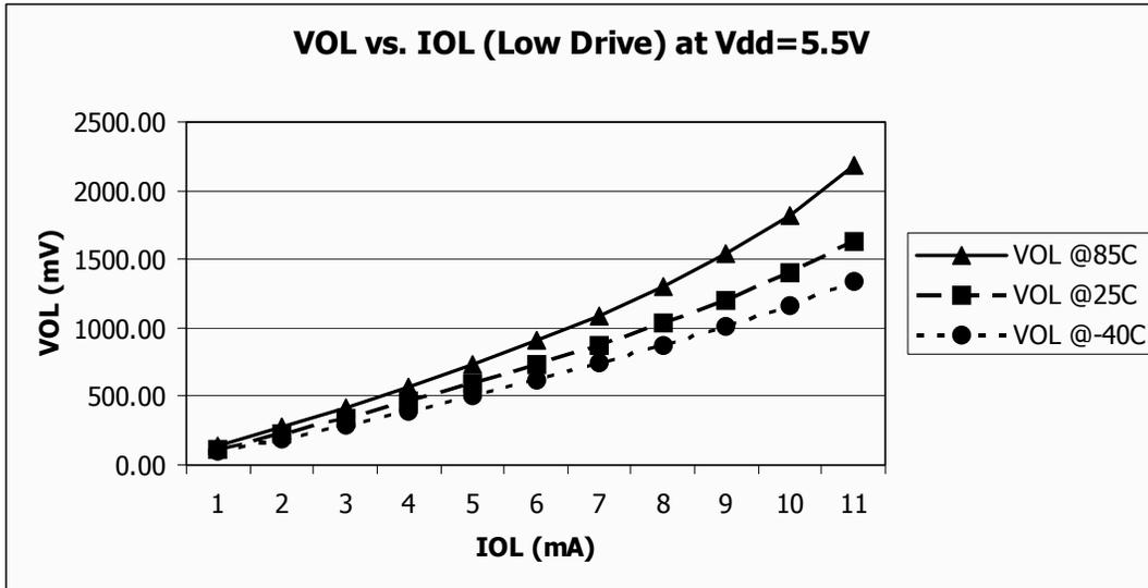
Figure 13. Typical  $V_{OL}$  vs.  $I_{OL}$
