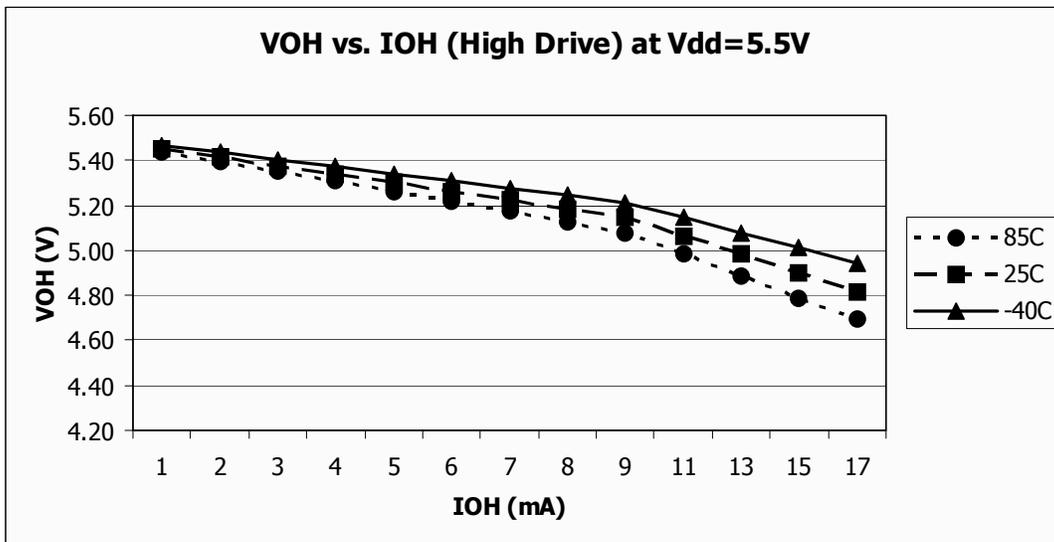
Figure 18. Typical  $I_{OH}$  vs.  $V_{DD}-V_{OH}$
