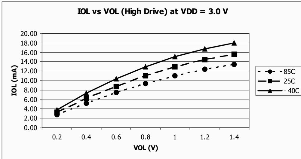
Figure 26. Typical I<sub>OL</sub> vs. V<sub>OL</sub>
