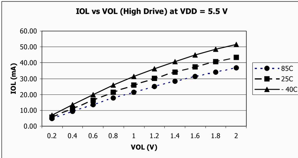
Figure 24. Typical  $I_{OL}$  vs.  $V_{OL}$
