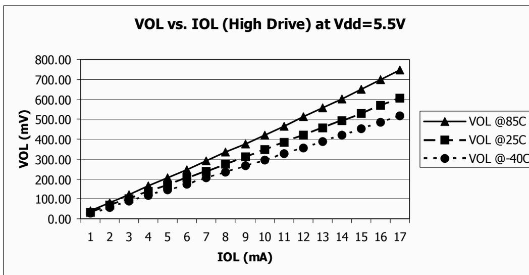
Figure 12. Typical V<sub>OL</sub> vs. I<sub>OL</sub>
