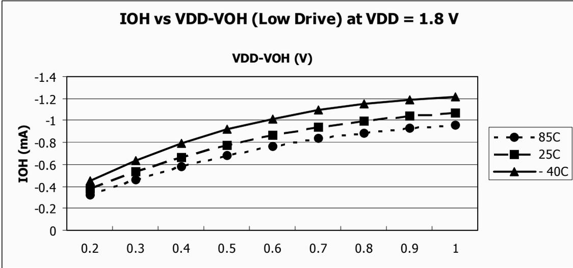
Figure 23. Typical  $I_{OH}$  vs.  $V_{DD}-V_{OH}$
