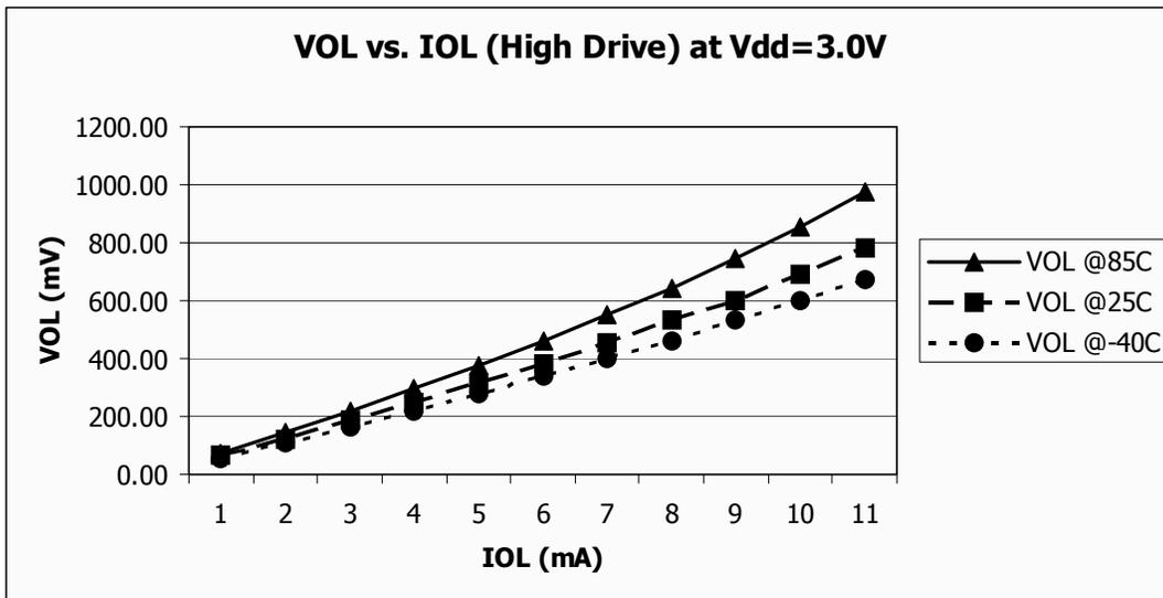
Figure 14. Typical  $V_{OL}$  vs.  $I_{OL}$
