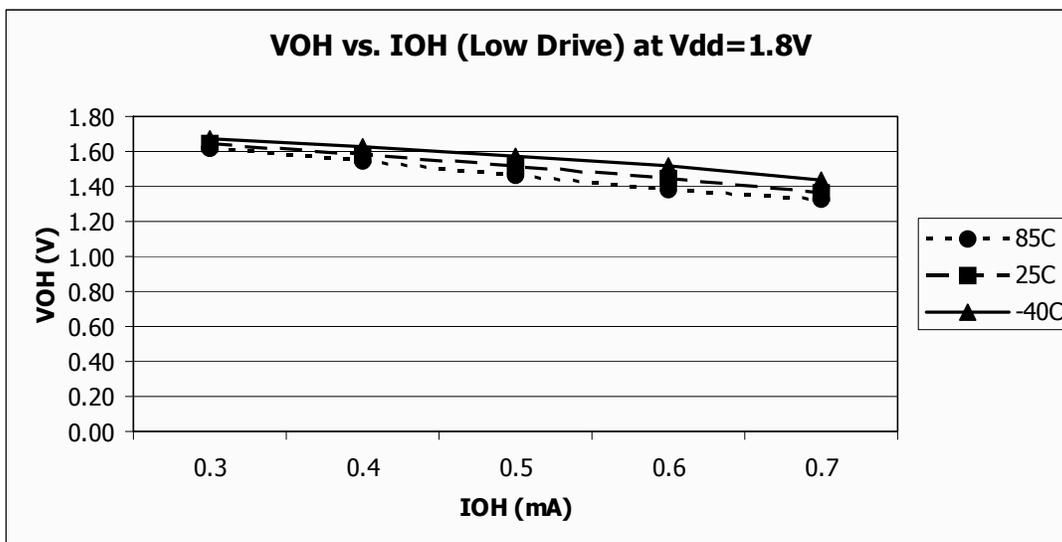
Figure 11. Typical V<sub>OH</sub> vs. I<sub>OH</sub>
