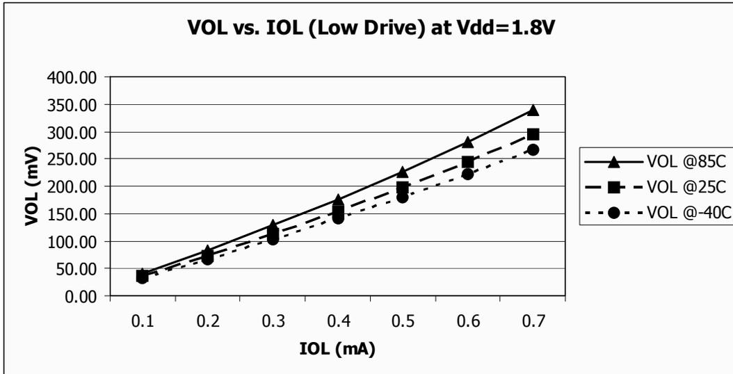
Figure 17. Typical  $V_{OL}$  vs.  $I_{OL}$
