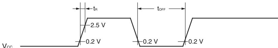
Note: A sudden change of power supply voltage may activate the power-on reset function. When changing the power supply voltage during the operation, set the slope of rising to a value below within 30 mV/ms as shown below.
