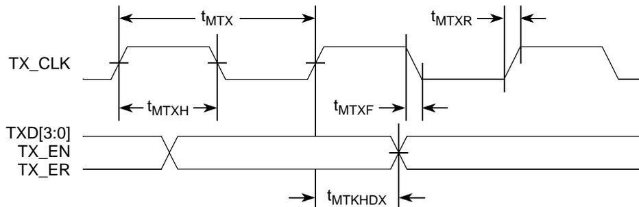
**Figure 10. MII Transmit AC Timing Diagram**
