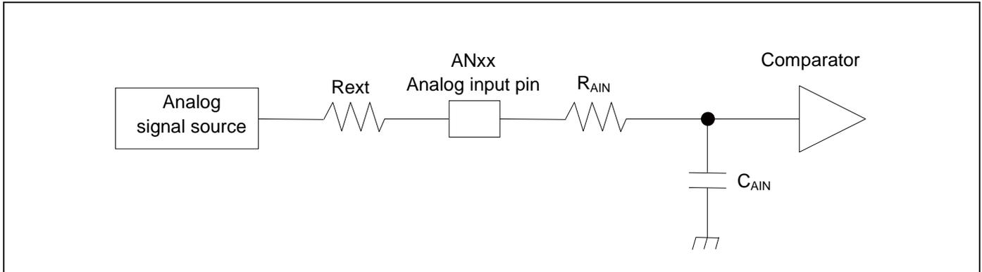
(Equation 1)  $T_s \geq (R_{AIN} + R_{ext}) \times C_{AIN} \times 9$
