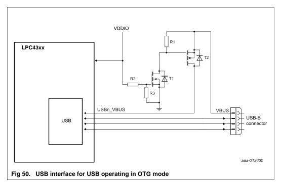
**Remark:** In OTG mode, it is important to be able to detect the VBUS level and to charge and discharge VBUS. This requires adding active devices that disconnect the link when VDDIO is not present.
