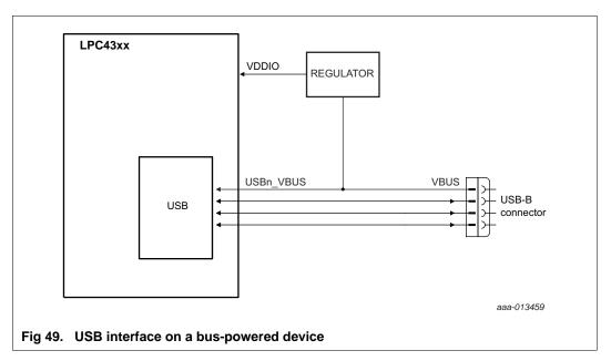
**Remark:** If the VBUS function of the USB1 interface is not connected, configure the pin function for GPIO using the function control bits in the SYSCON block.
