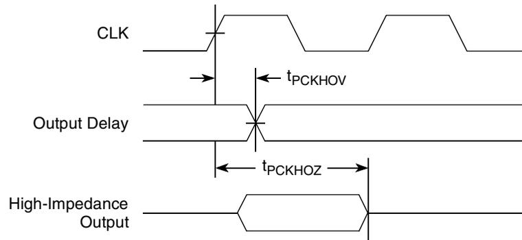
Figure 38. PCI Output AC Timing Measurement Condition
