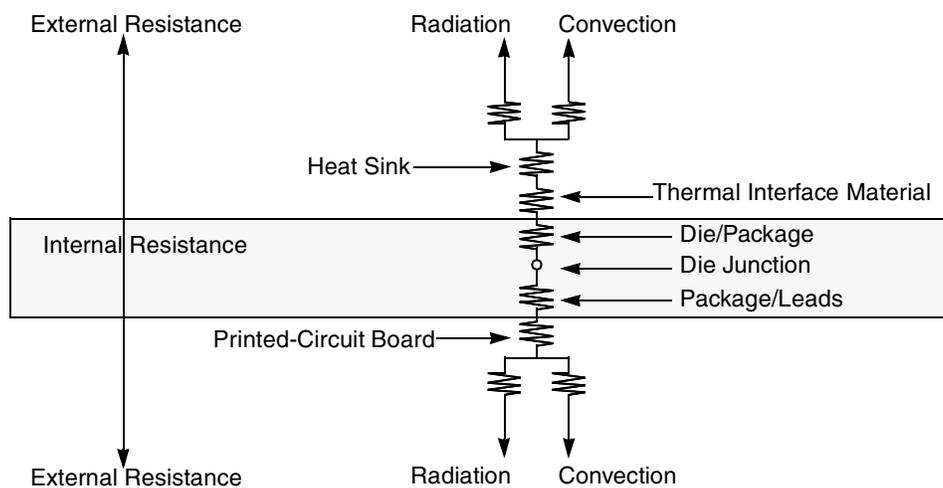
(Note the internal versus external package resistance)
