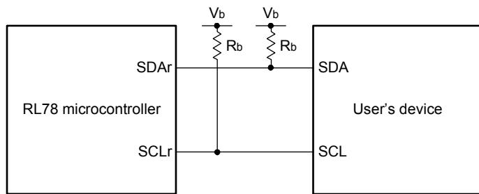
**Simplified I<sup>2</sup>C mode serial transfer timing (during communication at different potential)**
