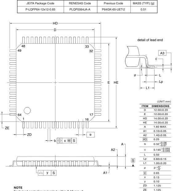
Each lead centerline is located within 0.13 mm of its true position at maximum material condition.
