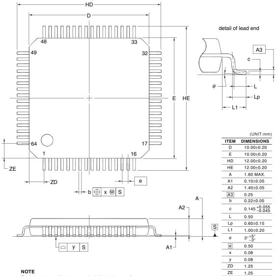
Each lead centerline is located within 0.08 mm of its true position at maximum material condition.
