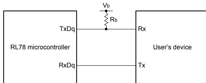
**UART mode bit width (during communication at different potential) (reference)**
