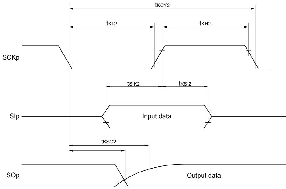
**CSI mode serial transfer timing (slave mode) (during communication at different potential)**
