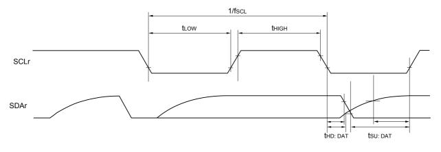
Remark 1. Rb[Ω]: Communication line (SDAr) pull-up resistance, Cb[F]: Communication line (SDAr, SCLr) load capacitance
