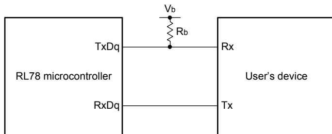
**UART mode bit width (during communication at different potential) (reference)**
