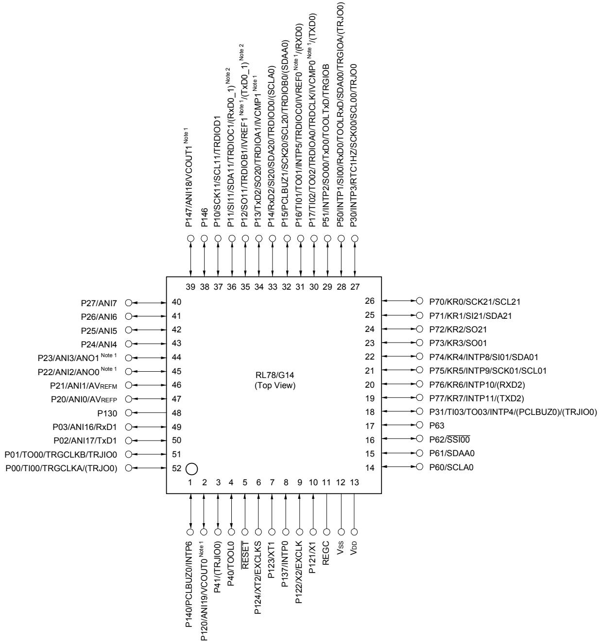
**Caution** Connect the REGC pin to Vss pin via a capacitor (0.47 to 1  $\mu$ F).
