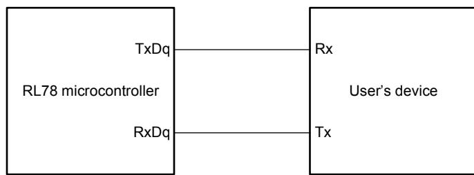
**UART mode bit width (during communication at same potential) (reference)**
