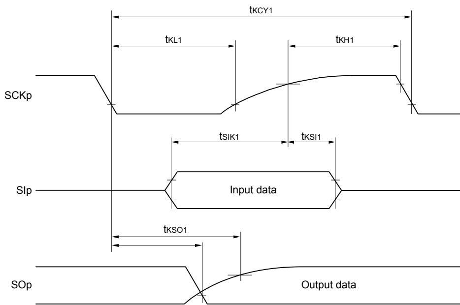
**CSI mode serial transfer timing (master mode) (during communication at different potential)**
