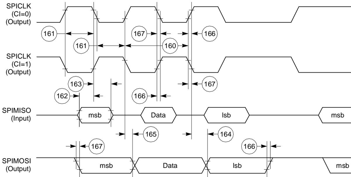
Figure 56. SPI Master (CP = 1) Timing Diagram
