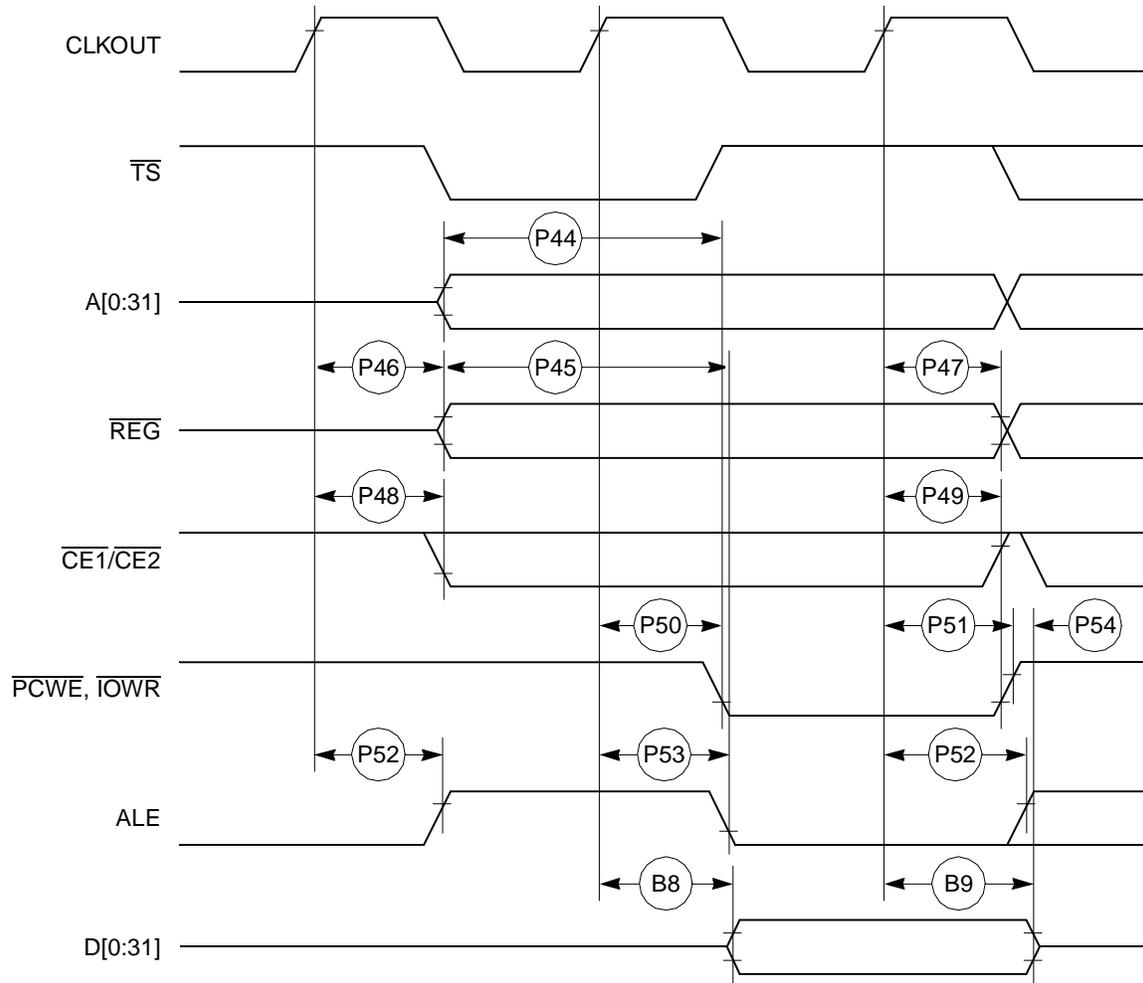
Figure 27. PCMCIA Access Cycles Timing External Bus Write
