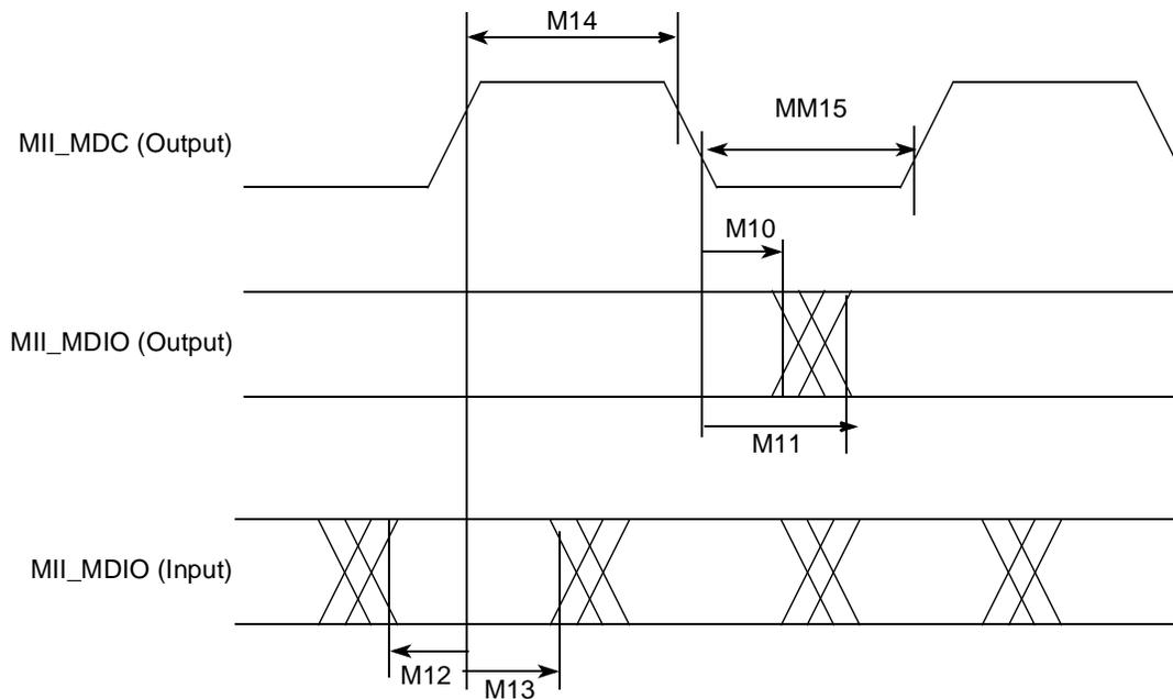
Figure 62. MII Serial Management Channel Timing Diagram
