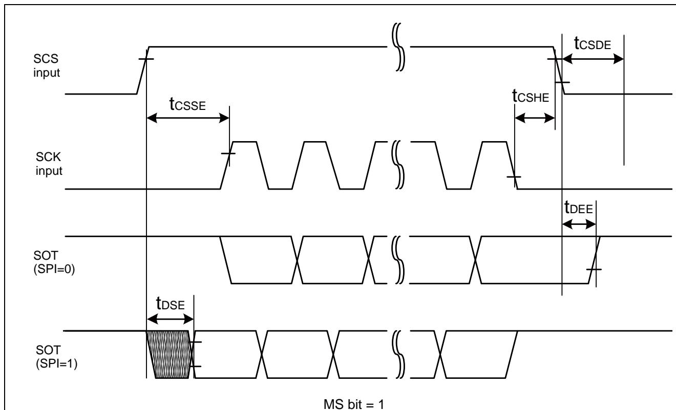
**High-Speed Synchronous Serial (SPI = 0, SCINV = 1)**
