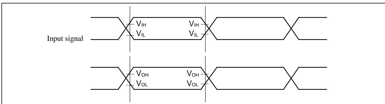
**When Using Synchronous Serial Chip Select (SCINV = 1, CSLVL = 0)**
