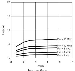
$I_{CCL} - V_{CC}$   $T_A = +25^{\circ}C$ ,  $F_{MPL} = 16$  kHz (divided by 2) Subclock mode with the external clock operating
