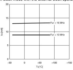
$I_{CCS}-T_A \\ V_{CC}=5.5~V,~F_{MP}=10,~16~MHz~(divided~by~2) \\ Main~sleep~mode~with~the~external~clock~operating$
