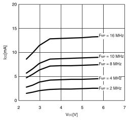
$I_{CCS}-V_{CC} \\ T_A=+25^{\circ}C,\, F_{MP}=2,\,4,\,8,\,10,\,16\,MHz \mbox{ (divided by 2)} \\ Main sleep mode with the external clock operating}$
