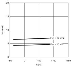
$I_{CCL}-T_A \\ V_{CC}=5.5 \text{ V, } F_{MPL}=16 \text{ kHz (divided by 2)} \\ \text{Subclock mode with the external clock operating}$
