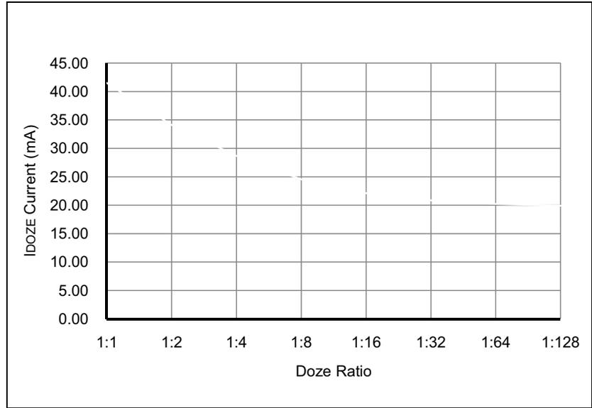
**FIGURE 32-6: TYPICAL/MAXIMUM I<sub>DD</sub> CURRENT @ V<sub>DD</sub> = 3.3V**
