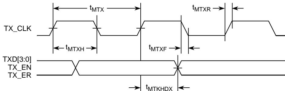
**Figure 9. MII Transmit AC Timing Diagram**
