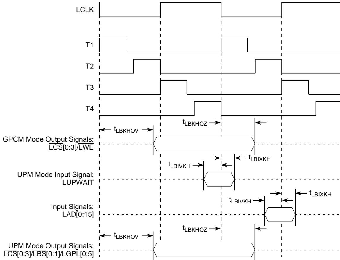
Figure 26. Local Bus Signals, GPCM/UPM Signals for LCRR[CLKDIV] = 4
