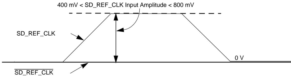
Figure 41. Single-Ended Reference Clock Input DC Requirements
