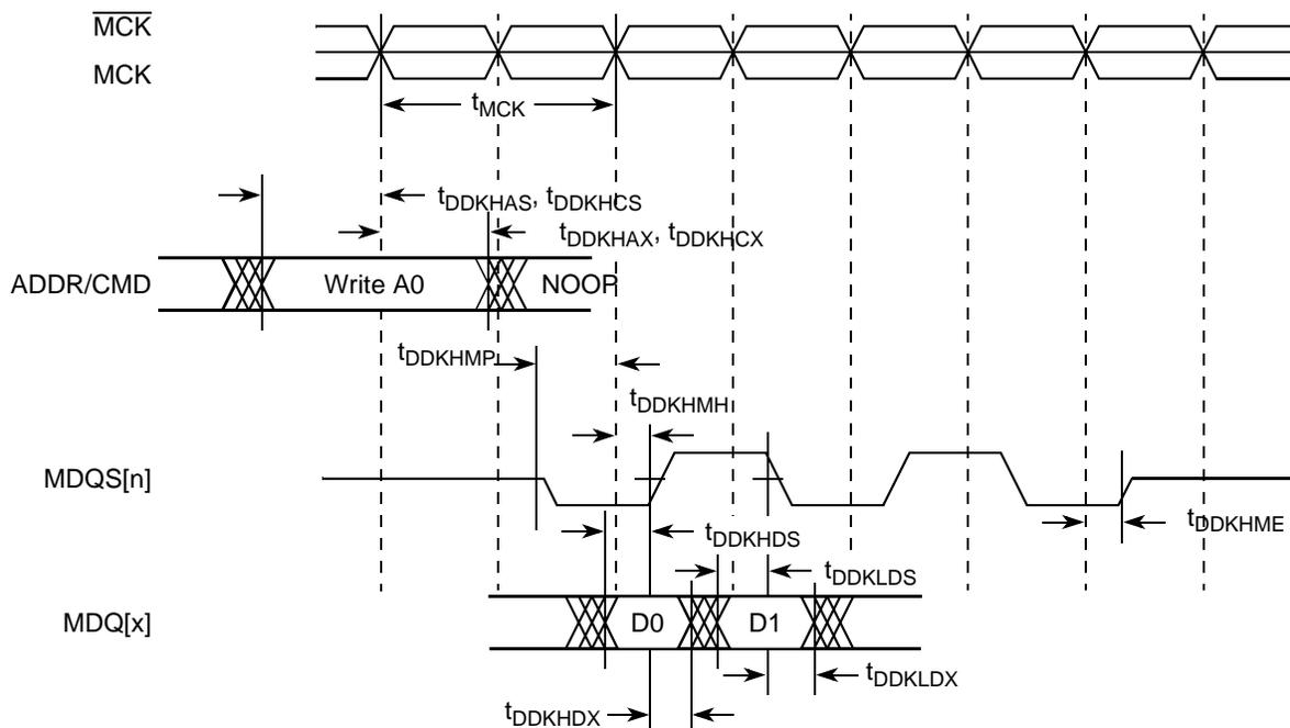
Figure 7. DDR and DDR2 SDRAM Output Timing Diagram
