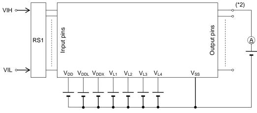
\*1: Input logic circuit to determine the specified measuring conditions.\*2: Measured at the specified output pins.
