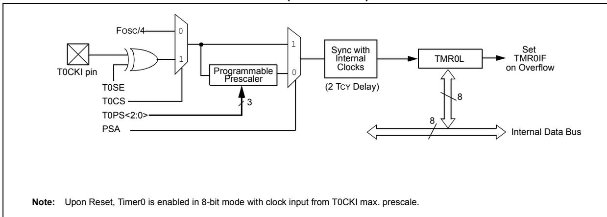
**FIGURE 12-2: TIMER0 BLOCK DIAGRAM (16-BIT MODE)**
