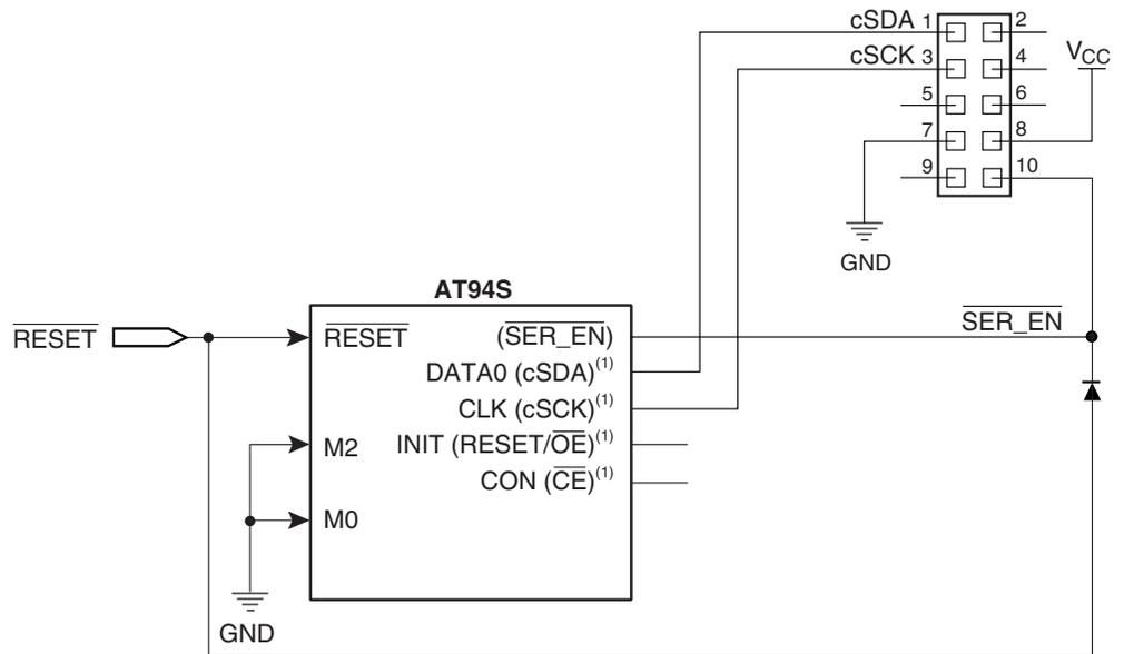
Note: 1. Configurator signal names are shown in parenthesis.
