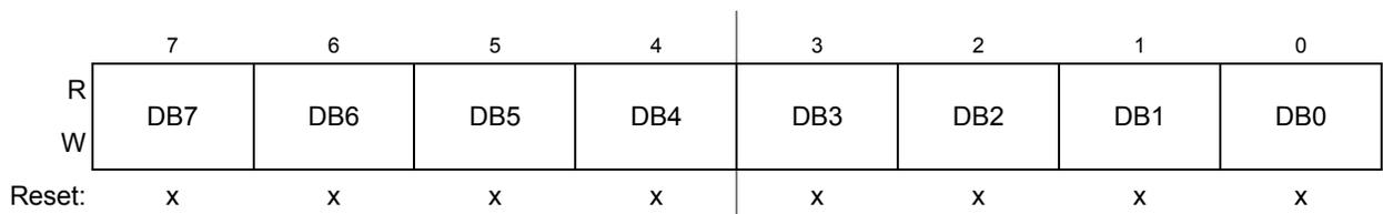
Figure 13-34. Data Segment Registers (DSR0–DSR7) — Extended Identifier Mapping
