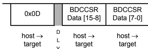
16-bit write to the BDCCSR register. No ACK pulse is generated. Writing to this register can be used to configure control bits or clear flag bits. Refer to the register bit descriptions.
