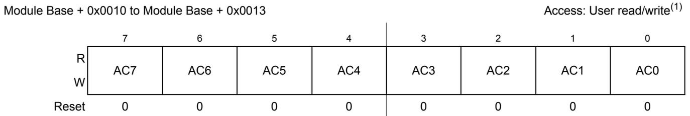
**Figure 13-20. MSCAN Identifier Acceptance Registers (First Bank) — CANIDAR0–CANIDAR3**
