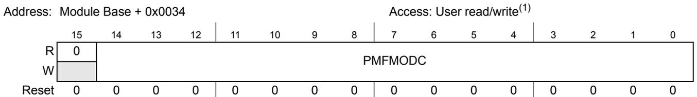
**Figure 15-37. PMF Counter Modulo C Register (PMFMODC)**
