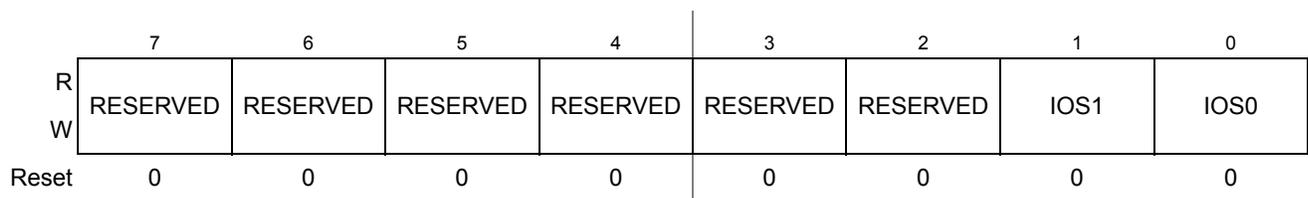
Figure 12-4. Timer Input Capture/Output Compare Select (TIOS)
