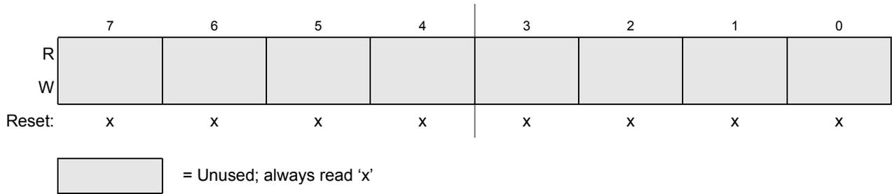
Figure 13-32. Identifier Register 2 — Standard Mapping
