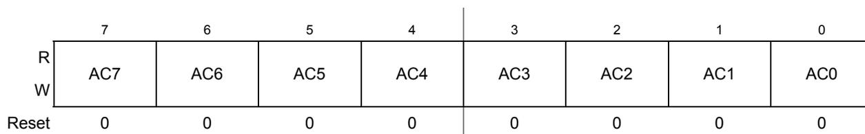
**Figure 13-21. MSCAN Identifier Acceptance Registers (Second Bank) — CANIDAR4–CANIDAR7**
