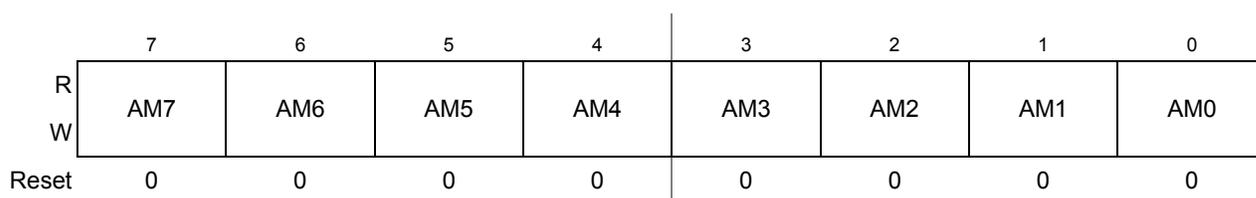
**Figure 13-22. MSCAN Identifier Mask Registers (First Bank) — CANIDMR0–CANIDMR3**
