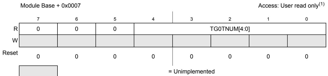
**Figure 14-10. Trigger Generator 0 Trigger Number Register (TG0TNUM)**
