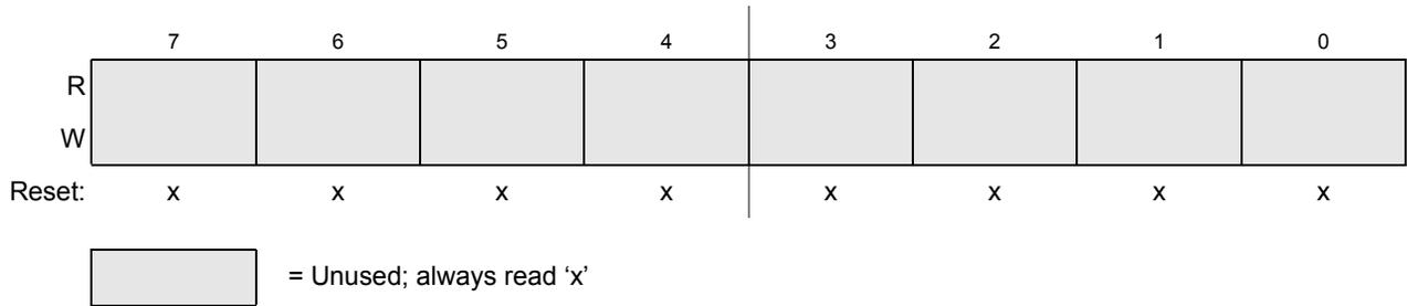
Figure 13-33. Identifier Register 3 — Standard Mapping
