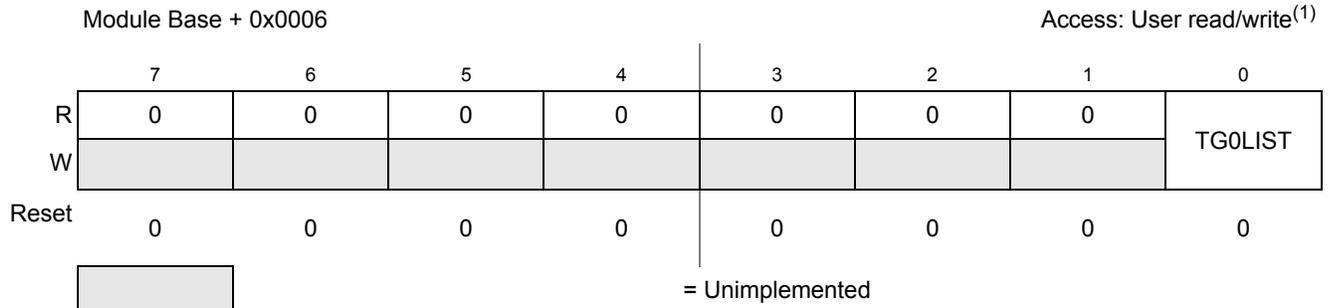
**Figure 14-9. Trigger Generator 0 List Register (TG0LIST)**
